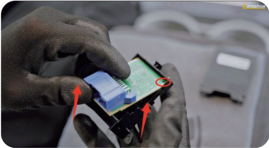
17. Lift the electronic board upward (pay attention to the alignment pin).
