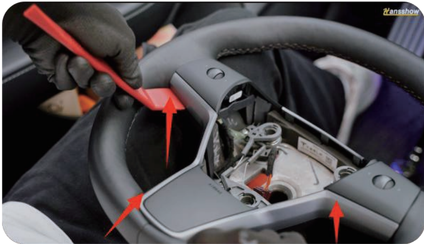
11. Use a trim removal tool to lever open the center trim panel of the steering wheel.
