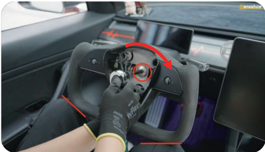
27. Use an H10 socket and an adjustable wrench to tighten the securing screws clockwise (If working alone, you can use your knees to support both sides of the steering wheel).
