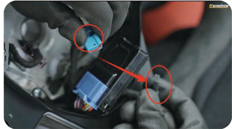
22. Disconnect the heating connector for ease of storing the control box in its subsequent location.
