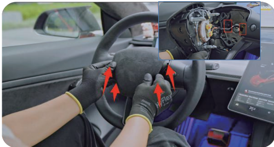
3. Lift the airbag assembly upward (Note that the wiring harness is still connected)
