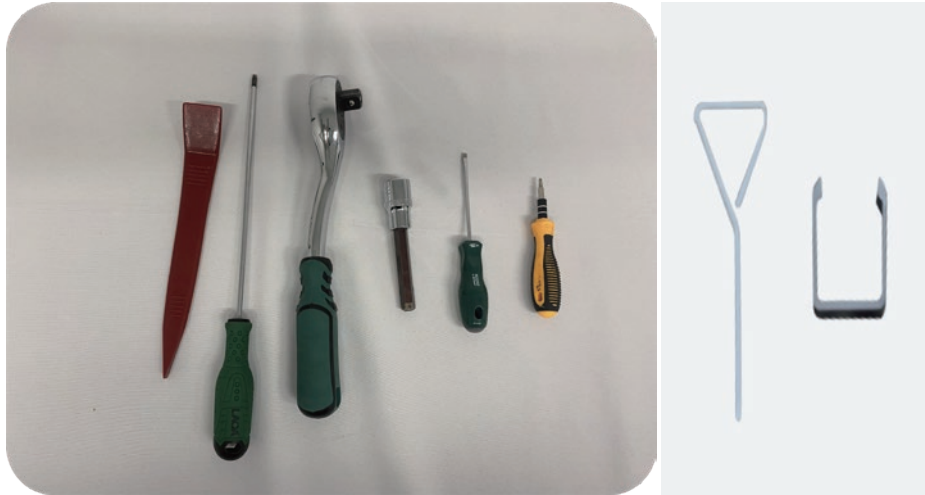
1. Disassembly and Assembly Tools: Trim removal, T20 and T10 Screwdriver, Socket Wrench, H10 Socket, Phillips Screwdriver, Additional Tool (Right)
