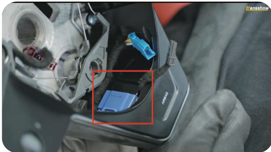
23. First, press the control box downwards at an angle and then press it upwards to secure it in place.
