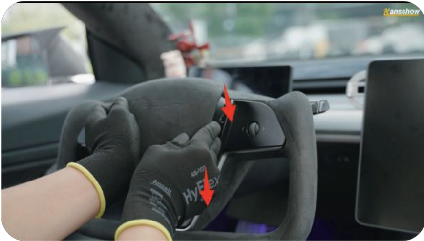
27. Align the airbag with the three holes and press it into place.
