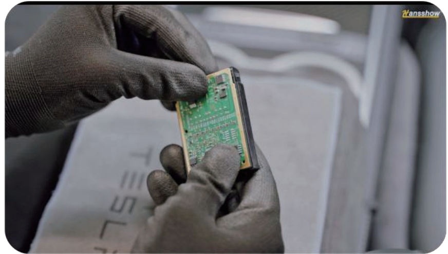
18. Install the removed factory chip onto the small control box.
