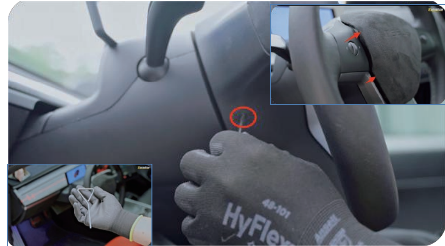
2. Insert the provided specialized tool into the small holes on both the left and right sides of the steering wheel to remove the airbag cover
