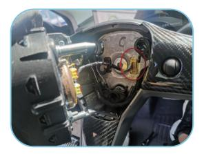
11. Finally, insert the airbag plug, and insert the airbag into the spring bayonet.
