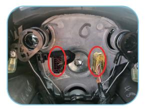
5. Take out the airbag and pull out the airbag plug and steering wheel plug.
