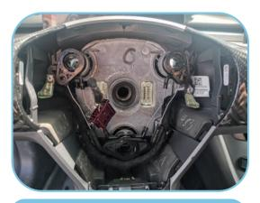
8. Then pull out the steering wheel. If the steering wheel is  $t_0$  o tight, shake it left and right and pull it out slowly.
