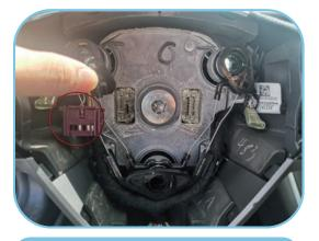
6. Note that the steering wheel plug must be pulled out to avoid pulling out the hairspring.
