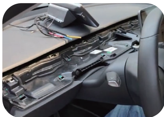
10. Remove the entire central control panel
