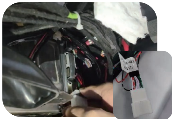
5. Connect the OBD plug to the female plug of the Y-type plug provided by us
