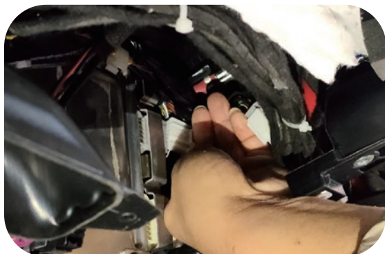
6. Insert the connected plug into the original position of the OBD plug
