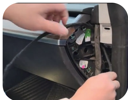
9. Then thread the wire harness to this position, as shown in the figure
