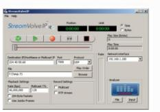
**Provisioned for Transport** Streams to be Sent to Single or Multiple UDP/IP, TCP/IP & RTP/IP Addresses.
