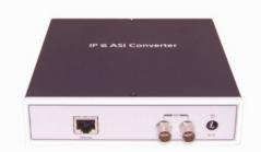
The CTDK is an ASI to IP or IP to ASI Converter for Bidirectional SPTS or MPTS Transport Streams over High-Speed IP Backbones.
