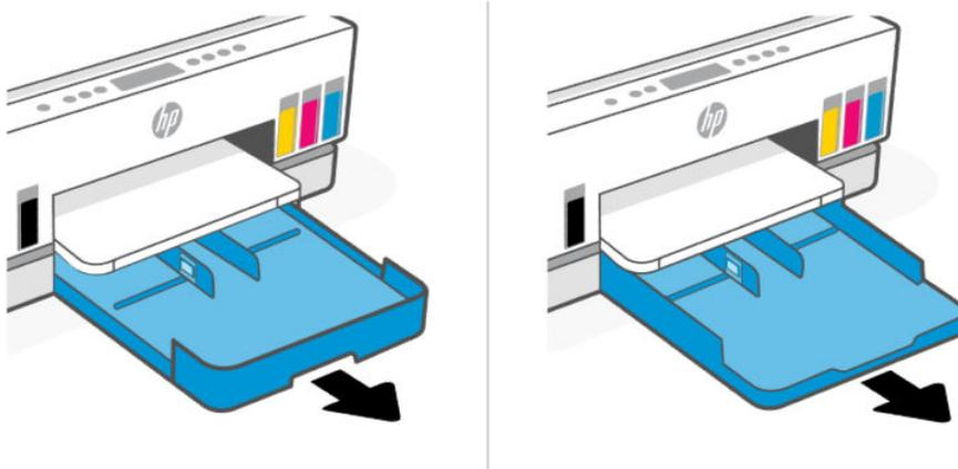
2. Press and hold the button on the paper-width guide, and then slide the guides to the edges of the tray.
