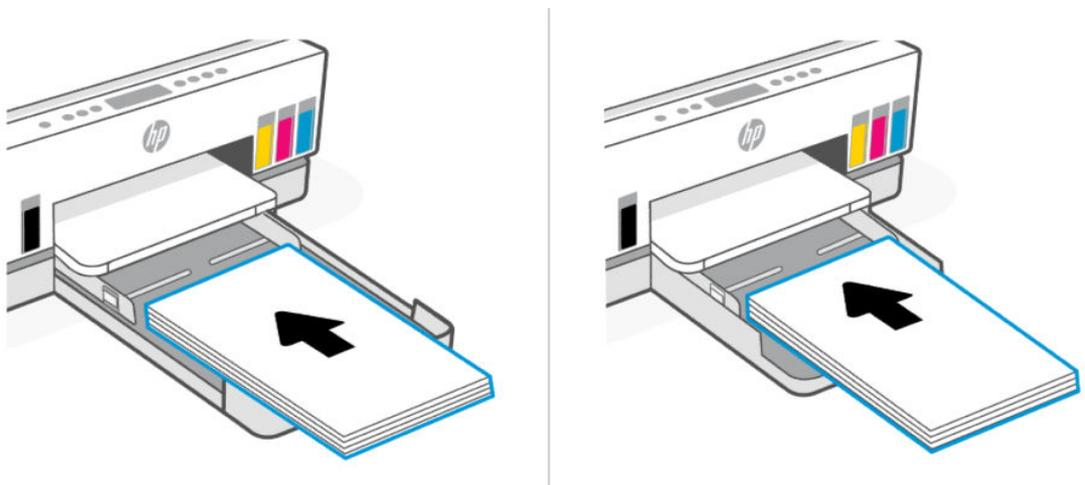
Make sure the stack of paper is aligned with the appropriate paper size lines in the tray. Also, make sure the stack of paper does not exceed the stack-height marking in the tray.
