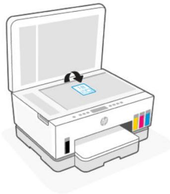
7. Press the copy button that is blinking or lit to copy the other side.
