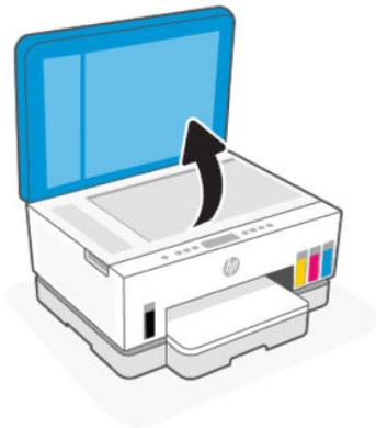
2. Clean the scanner glass and lid backing by using a dry and soft, lint-free cloth. Spray the cloth with a mild glass cleaner and clean **only** the glass.
