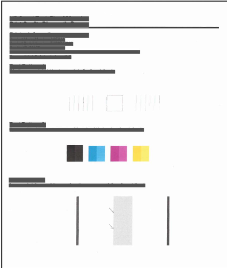
2. If the diagnostic page shows streaks or missing portions of the color and black boxes, then automatically clean the printheads.
