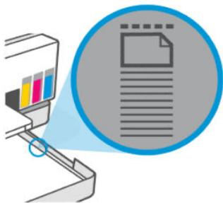
5. Adjust the paper-width guides until they touch the edges of the stack of paper.
