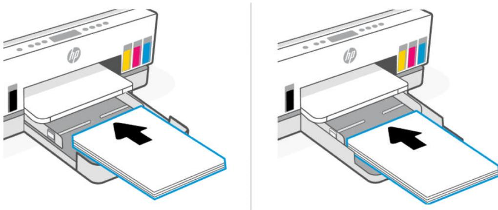
Make sure the stack of paper is aligned with the appropriate paper size lines in the tray. Also, make sure the stack of paper does not exceed the stack-height marking in the tray.
