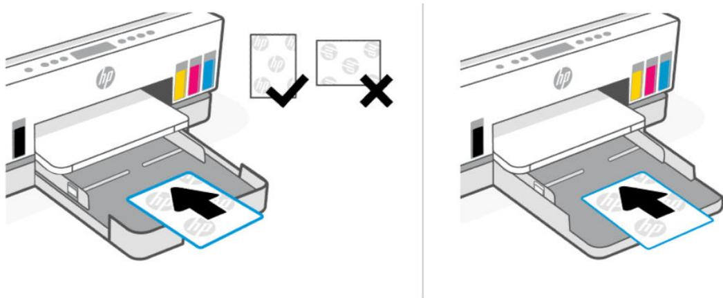
Make sure the stack of paper is aligned with the appropriate paper size lines in the tray. Also, make sure the stack of paper does not exceed the stack-height marking in the tray.
