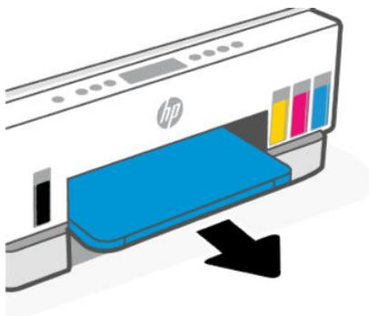
3. Remove the duplexer plate. Do this by carefully reaching inside the gap where the trays were and pulling out the plate.
