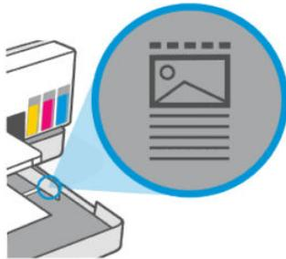
4. Adjust the paper-width guides until they touch the edges of the stack of paper.
