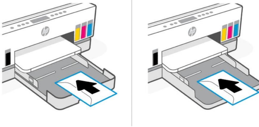
Make sure the stack of paper is aligned with the appropriate paper size lines in the tray. Also, make sure the stack of paper does not exceed the stack-height marking in the tray.
