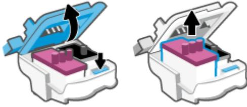
5. Clean the printhead contacts and printer contacts.
