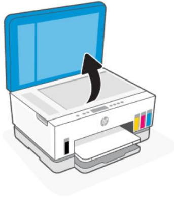
2. Load the original print-side down on the scanner glass (aligned to the indicated corner).
