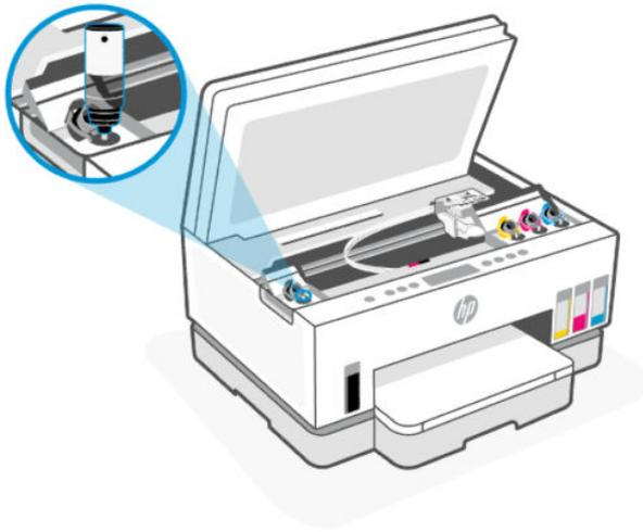
5. Let the ink drain into the tank until the tank is full.
