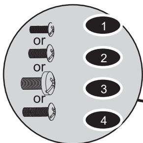
Use M8M5 adapter **A2** with 5mm x 12mm screw **2** or 5mm x 20mm **4** screw if TV has 8mm inserts. Insert **A2** into 8mm insert on back of TV then follow steps below.
