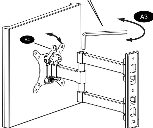
Flat panel can be leveled (+/- 3 degrees) as needed. *If Philips screw is tensioned too tight it will be difficult to adjust leveling.*
