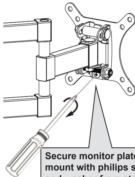
Secure monitor plate to mount with philips screw and washer from step 1. Do not over-tighten screw.
