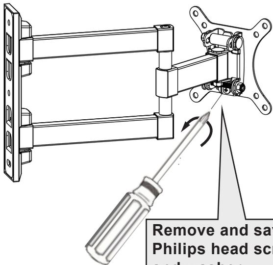
Remove and save Philips head screw and washer. Screw and washer will be used to reattach monitor plate in Step 4
