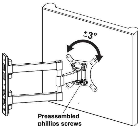
The elbow points can be adjusted by using the Allen Key **A3**.
