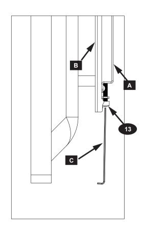
Secure allen security screws on monitor plate with security allen key.
