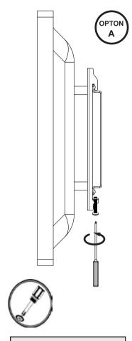
Secure pre-installed screws on monitor plate to wall plate.
