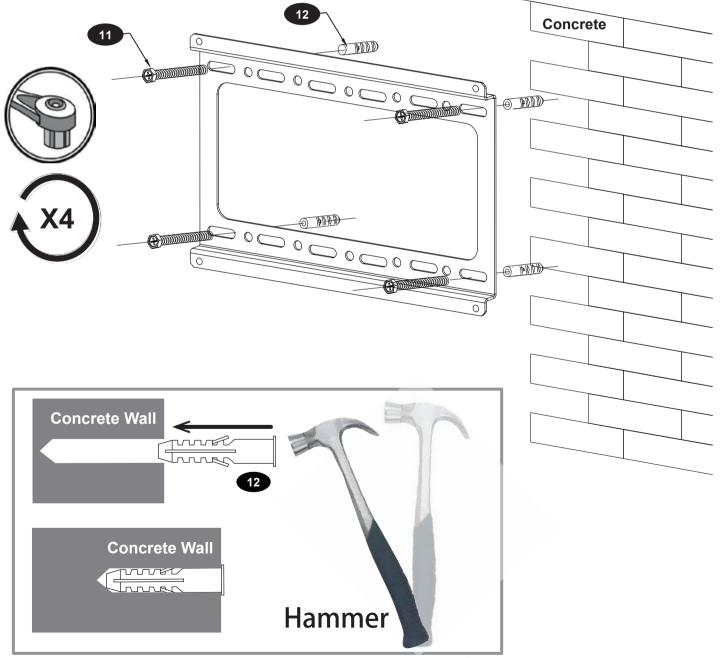
Insert wall anchors gently into concrete wall with hammer if necessary
