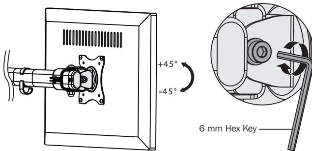
It may be necessary to slightly loosen or tighten the adjustment screw, depending on the weight of display installed.
