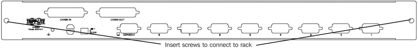
Fasten the rackmount brackets to the rack with user-supplied screws to install in a rack.
