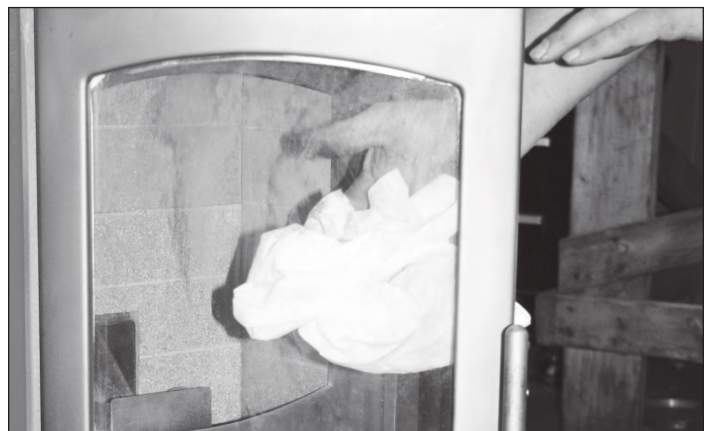
Figure 31: Wipe glass and inspect gasket
