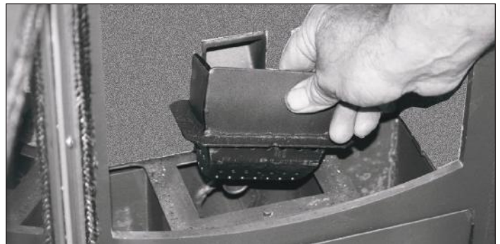
Figure 30: Fire pot clean
