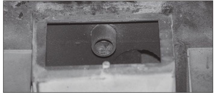
Figure 34: Remove ash from igniter tube (underneath firepot)
