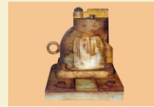
GAUGE WITH OXIDATION
