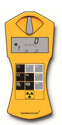
• Press the button I to switch GAMMA-SCOUT® to the pulse count mode. The display will show the pulse symbol. Counting will not have started yet. Pressing the button I a second time will start the counting without pre-setting the measuring time.
