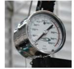
The HP gauge displays the pressure on the high-pressure water line. This allows the operator to see the actual pressure supplied to the cutting head and assists in troubleshooting.
