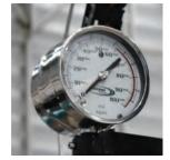
The HP gauge displays the pressure on the high-pressure water line. This allows the operator to see the actual pressure supplied to the cutting head and assists in troubleshooting.
