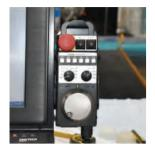
The MPG allows to manually wind forward or backward through a cutting path. This enables the operator to find the exact point along a cutting path from which to re-start cutting after a stoppage, or to accurately locate a pre-cut part.
