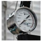
The HP gauge displays the pressure on the high-pressure water line. This allows the operator to see the actual pressure supplied to the cutting head and assists in troubleshooting.
