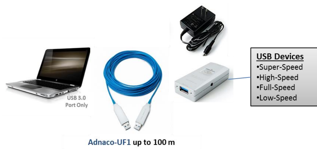
Fig.1 Usage Scenario for the full set of USB protocols
