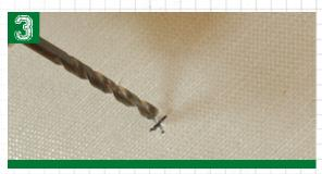
Using your drill with the 3/8" bit, drill the hole for your rubber tee starting from the back of the turf.
