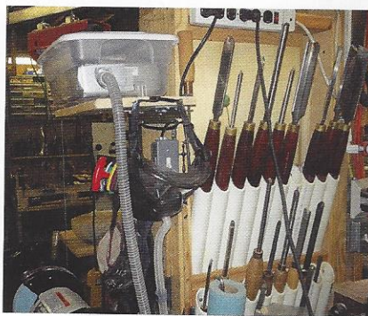
The unit is mounted on a shelf near the lathe and turning tools. The switch is positioned just below the unit.
