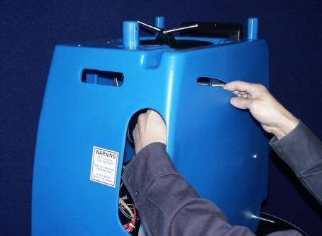
8. With the rod below the groove you can see the wall bulge slightly. This is normal.
