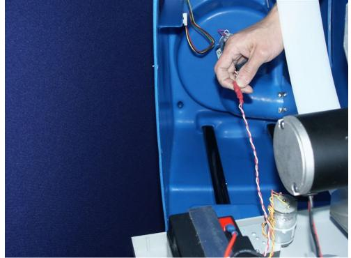
11. The blue body can now be removed completely. Note that the remote control receiver (Star only) and carousel motor stay with the blue body. All other components, including the battery, are on the base.
