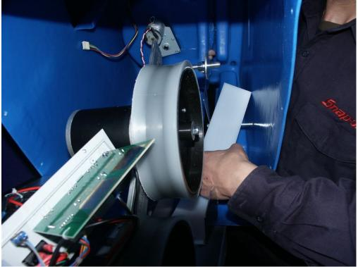
19. You will need to guide the motor carrying arm as well as the threaded rod back in their place. Note that there is one or two large washers on the inside of the wall. If these fell during previous steps, be sure to replace them before proceeding.
