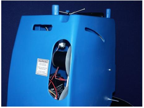
9. The blue body of the machine can now be pulled out carefully. There is still two wires to disconnect to free it (see next step).
