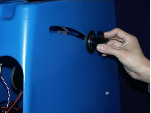
7. Disengage the threaded rod by pulling the inner arm away from the wall (left hand in picture) and pulling the plastic wall in the opposite direction (right hand in the picture). Now nudge the blue body upward so that the threaded rod will be below the groove.
