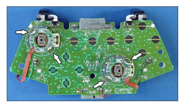
(6)Use the Double Sided Adhesive tape to fix the cable ,after that install the left and right analog sticks, place the PCB to the X1 controller top shell ,then plug the flat soft cable to the socket (As shown on the picture)
