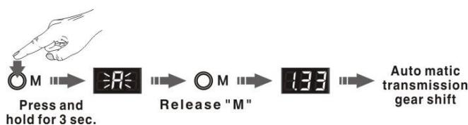
Press and hold the M button on the device for 3 seconds, wait the digit tube shows **H** and blinks, now release the M button, the setting is completed , the gear shifter is changed from + and – mode control to manual control.
