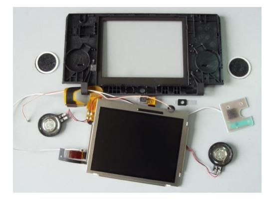
21.roll up the flat cable and remove it from the shell.
