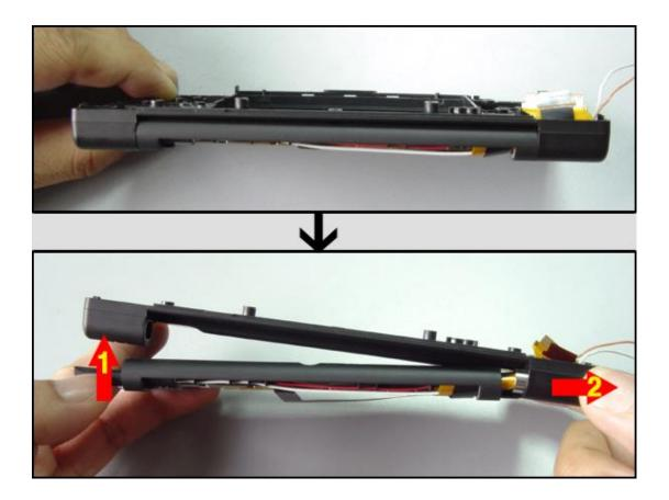
16.Push the ring from the console's lower part of LED panel cover to the console's upper part of LED panel cover
