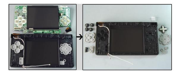
12.Remove those rubber tabs and screws for moving apart the upper console's bottom part from the shell.
