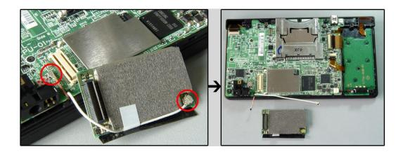
10.Follow the arrow direction 1 to unfold the socket then slowly to take out the flat cable (follow the arrow direction 2), and do the same job for the back of this part.
