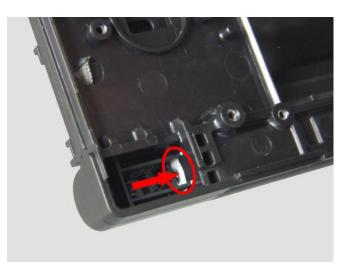
15.Follow the direction of arrow 1 to push up the console's lower part of LED panel cover, and slowly pull out the shell (follow the direction of arrow 2).
