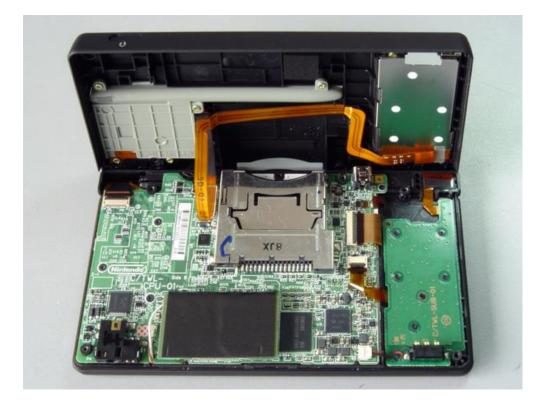
5.Unplug the cable to let the bottom part of lower shell apart from the pcb.
