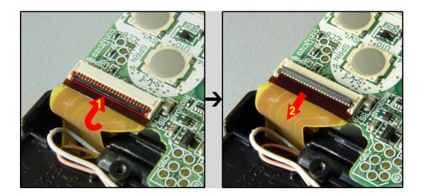
11.As shown on the picture, remove the PCB from the console's lower part of LED panel cover and take out all the parts.
