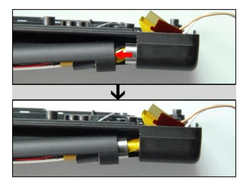
17.Put the flat cable to the notch (arrow indicates) then slowly pull out the cable from the notch (Picture C), now two parts is separate (Picture D).
