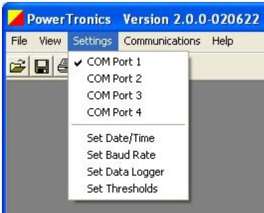
The "Settings" menu contains items that allow the user to specify certain settings for communication between the software and the PQR device. The menu also provides an interface for setting the PQR device parameters.
