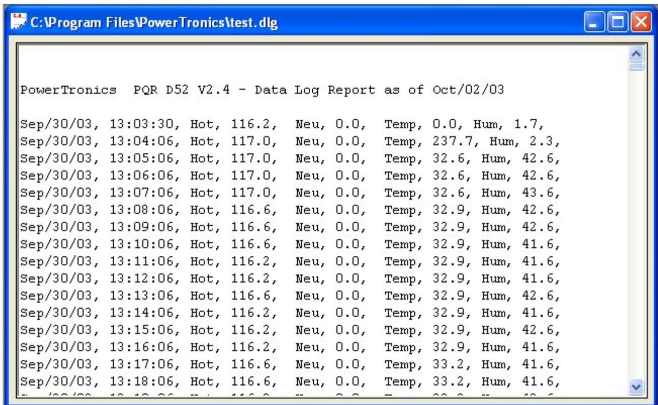
This is the text report showing the Date and Time of the reading, the voltage on each of the Hot and Neutral Lines as well as the readings from the Temperature and Humidity sensors.
