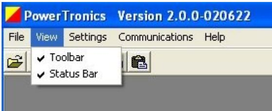
The "View" menu contains items used to control what tools are visible and available to the user in the main program window.
