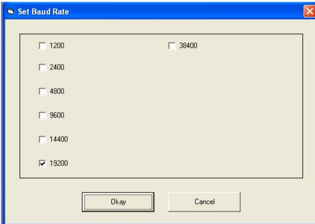
The "Set Baud Rate" menu option allows the user to specify the data rate to be used when communicating with the device. The program will display a dialog box with the six valid baud rates to select from: 2400, 4800, 9600, 14400, 19200 and 38400. After selecting the desired baud rate, pressing the "Okay" button will instruct the program to set the device baud rate. This process may take a few seconds. The program baud rate setting will also be set to the selected setting.
