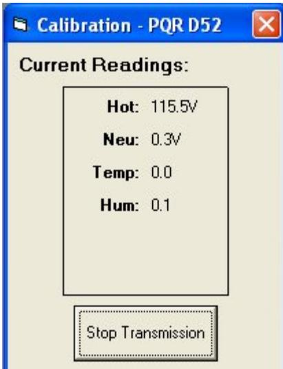
Selecting the "Calibration Mode" menu item will command the device to begin transmitting the current voltage readings to the computer. The voltage readings are then displayed in a special window. The voltage readings will be updated approximately once a second. No other command can be performed while the program is in calibration mode. To end the transmission, user must press the "Stop Transmission" button; otherwise, the transmission will automatically stop after about two minutes.
