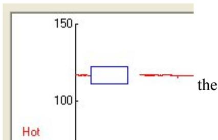
By holding down your Left Mouse Button you create a selection box. You can drag your mouse, and create a ZOOM Area around your data. When you release the mouse button, data in the ZOOM area is expanded to fill the screen area.
