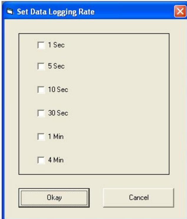
The "Set Data Logger" menu item allows the user to specify the device data logging rate, or the time in between data log samples. The user will be provided six choices: 1 second, 5 seconds, 10 seconds, 30 seconds, 1 minute, or 4 minutes. After selecting the desired logging interval, pressing the "Okay" button will instruct the program to set the device setting. This process may take a few seconds.
