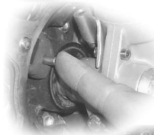
Recheck for a good closed time for the sensor before the putty hardens all the way.
