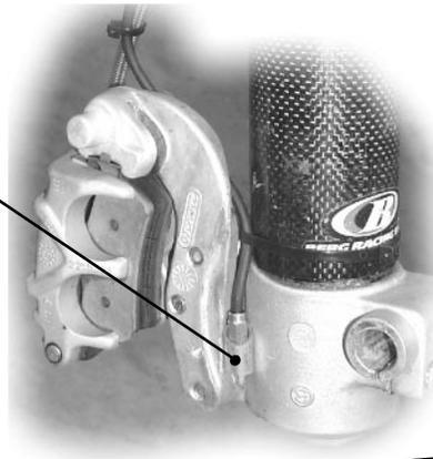
At the far right we bend a tab to 90°, Silicone the sensor then attach it to an existing screw.
