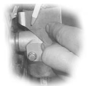
At the far right we mark a AutoCal tab where it will be hacksawed. A great way to attach the sensor is to prepare a tab as shown at the far right. This will work on almost every front end, plus it protects the sensor very well.
