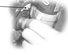
The CheckMate sensor bracket was designed to be hacksawed & bent into whatever shape is needed for your setup. Drill holes where required & either use the screws in the kit or use existing screws on the fork leg.
