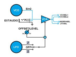
The figure left depicts how the VCO Sin<sup>2</sup> waveform inputs to a VCA to be enveloped by either LFO Reverse Sawtooth or Triangle waveforms.
