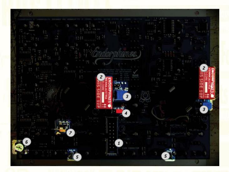
1. Dæpfer A-100 bus IDC-connector. We advise that you use the supplied 16-pin ribbon cable. Please ensure that the <u>red stripe</u> of the cable (the top pair of pins/wires) is connected to negative -12V rail when plugging the cable to your power distribution board. If the ribbon cable is connected backwards, the module might be destroyed. Please ensure twice before connecting since this is not covered under warranty.
