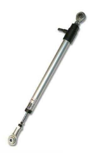
This mini position transducer is designed for direct absolute measurement and available in stroke length up to 150mm. The mini design is suitable for mounting in instruments or machines with limited space. An improved technique for making connection to resistance track (Double Trimming Technique) ensures track (double Trimming Technique) ensures the higher degrees of reliability and linearity, while multi-fingers wipers stabilize output signals, even in the most adverse working conditions.
