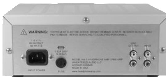
Plug the power cord into the amplifier, and the other end into a wall outlet. Connect the audio inputs of the HA-1 to your CD player or other source, using standard RCA-type audio interconnect cables. Note that the input connectors are color-coded, red for the right channel and white for the left.
