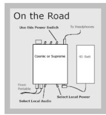
The Supreme can be operated on four Dcell batteries using the 4-D battery pack supplied with the amp. Alternate 5-6V. power supplies can also be used with the Supreme, and will connect into the same DC input. These are considered "local power", and the POWER switch on the rear of the amp should be set to LO-CAL. The power supply we recommend is the Supreme/Cosmic power supply, which connects into the 5-pin din connector (also used by the Base Station One, the ultimate power supply upgrade!).
