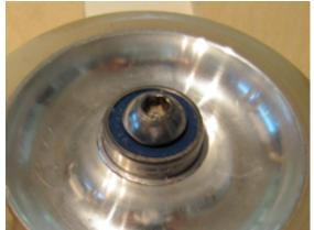
Now turn the wheel over. Take a front axle and put the second bearing on the axle followed by the bearing spacer. From the top of the wheel, slide the axle with the spacer and the bearing inside the bearing at the bottom of the wheel. This lines up the bearings and the spacer and prevents the spacer from tipping over while you are tapping. Now take the socket and tap in the top bearing using the same process.
