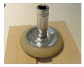
If the bearing tilts a bit, tap on the high side to level it out. **Always keep the socket in between the hammer and the bearing**. This is to avoid hitting the center rim of the bearing. Keep tapping the socket rotating your hammer strokes around the top edge of the socket until the bearing is completely inside the wheel.
