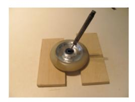
Take an old flathead screwdriver or a punch and insert it through the top bearing past the spacer. Hold it in an angle so the tip rests on the inner rim of the bottom bearing. Tap the punch or screwdriver with a hammer. Repeat this, switching sides on the bearing until it falls out of the wheel. If the bearing comes out easily without a lot of force, the bearing may still be usable. If excess force was needed, the bearing is likely damaged. Turn the wheel over and repeat the process above.
