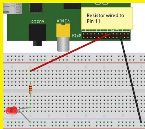
**Figure 2 - GPIO Test**
