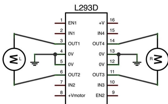
Motor rotation is controlled by IN\* and EN\*:
