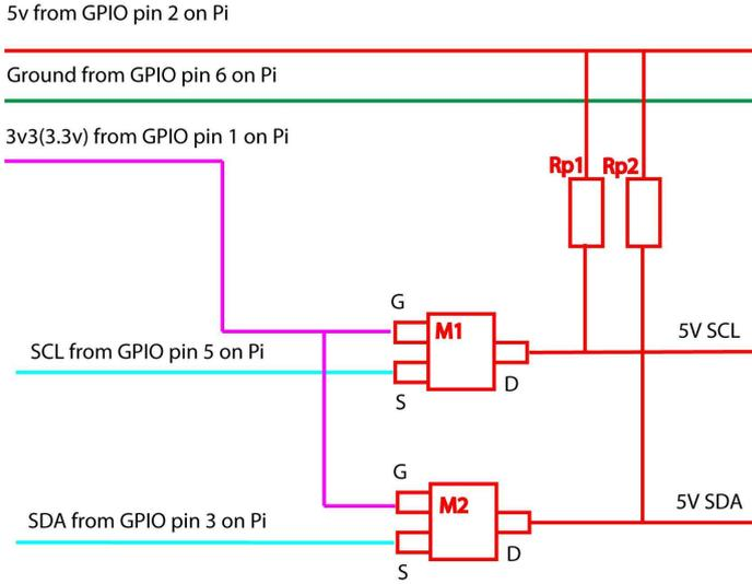
The purple line signifies 3.3V from the GPIO. This goes to the "Gate" on the MOSFET. The red line signifies the 5V supply. This is connected to the "Drain" of both of the MOSFETs via a "pull up" resistor. (In I<sup>2</sup>C the natural state of the bus is "low". When a current is applied to the bus via a pull up resistor, it temporarily pulls the signal up to an "on" or "high" condition).
