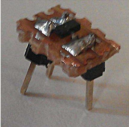
a small piece of stripboard, soldered the terminals of the MOSFET across these and then added some larger connectors to make it suitable for plugging into breadboard.
