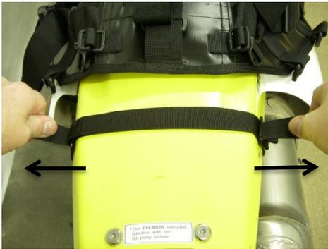
5. Thread Tension-O-Matic straps through rear buckles. Fig.5
