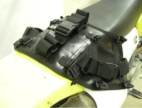
2. Place the Tension-O-Matic strap on the rear fender. Fig.2
