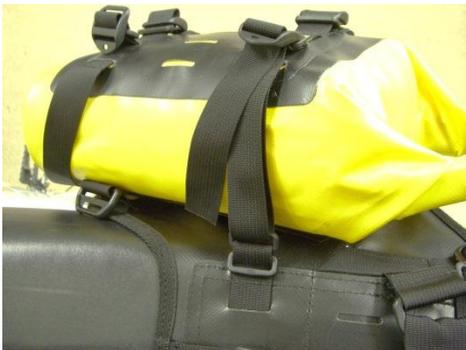
9. Thread the remainder of the webbing through the buckles on the mount and back to the buckles on the bag. Fig.12
