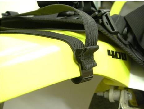
4. Pull the Tension-O-Matic strap away from the rear fender to tension straps.Fig.4
