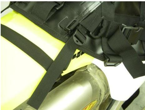
6. The Front mounting straps on the front of each side thread around the sub frame side tubes, below the side panels. Thread the webbing behind the sub frame from the bottom and out on the top. On the Exhaust side **BE Very Careful** (Yes, the webbing can be close to the exhaust header, the pipe can be very Hot.) Also we have designed the front straps so they can be replaced if they get melted or if you cut them too short. Left Side Fig. 6&7 Right Side Fig. 8&9
