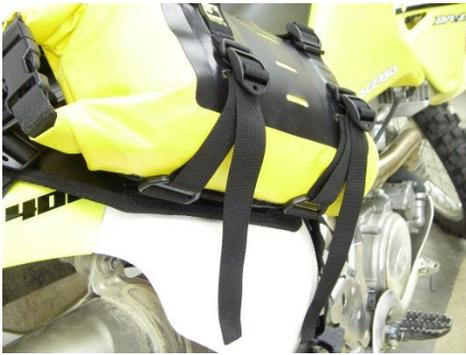
10. Attach the Wide strap across the outside of the Rolie Bag. Thread through the Handle Loop. Secure the excess web to the Flappy Strap Keepers. Fig.13
