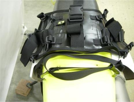
3. Spread the Gutter Hooks of the Tension-O-Matic mounting across the rear fender so the Gutter Hooks catch the bottom lip on each side of the rear fender. (You may have to grind the lip to make the Gutter Hooks fit tight. Fig.3
