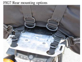
\*\*For more security thread the rear mounting straps through a rear rack or grab handle and through the 2"D-rings on the side compression straps and back to the buckle\*\* FIG7
