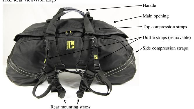
The Boulder Beta has handles under the side compression straps to help position the bag onto your motorcycle.
