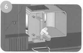
Insert the new lamp unit, paying attention to the orientation and direction of insertion. Ensure that the new unit is firmly seated.
