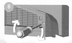
Replace the lamp cover by aligning it with the groove. Tighten the screw on the cover.
