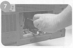
Replace the screw that secures the lamp, taking care not to overtighten.
