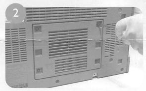
Locate the lamp door on the rear of the television; using a screwdriver, loosen and remove the four screws.
