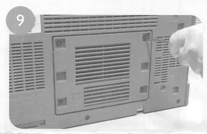
Tighten the screws on the lamp door.
