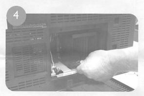
Remove the lamp cover duct by squeezing the clip and pulling it out.
