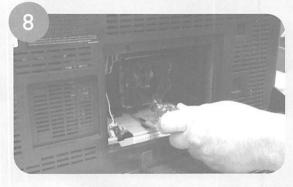
Replace the screw that secures the lamp, taking care not to overtighten.
