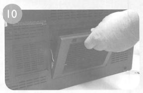
Replace the lamp door; replace and tighten the screw(s).
