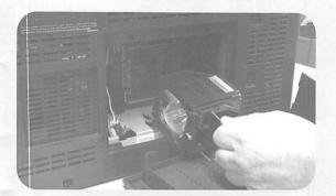
Remove the lamp unit from the television by grasping the handle and pulling it out. Dispose of lamp in accordance with disposal laws.
