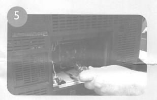
Using a screwdriver, remove the screw securing the lamp.
