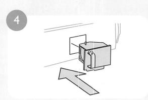
Insert the new lamp unit, paying attention to the orientation and direction of insertion. Ensure that the new unit is firmly seated. Tighten the screw securing the lamp cartridge, taking care not to overtighten.
