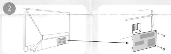
Using a Phillips head screwdriver, loosen and remove the two screws securing the outside lamp cover; remove the cover.
