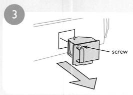
Loosen (but do not remove) the screw securing the lamp unit. Remove the lamp unit by grasping the handle and pulling straight out. Dispose of the lamp in accordance with disposal laws.
