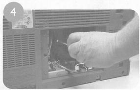
Using a screwdriver, loosen and remove the screw securing the lamp.
