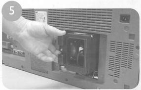
Remove the lamp unit from the television by grasping the handle and pulling it out. Dispose of lamp in accordance with disposal laws.
