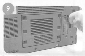
Tighten the screws on the lamp door.
