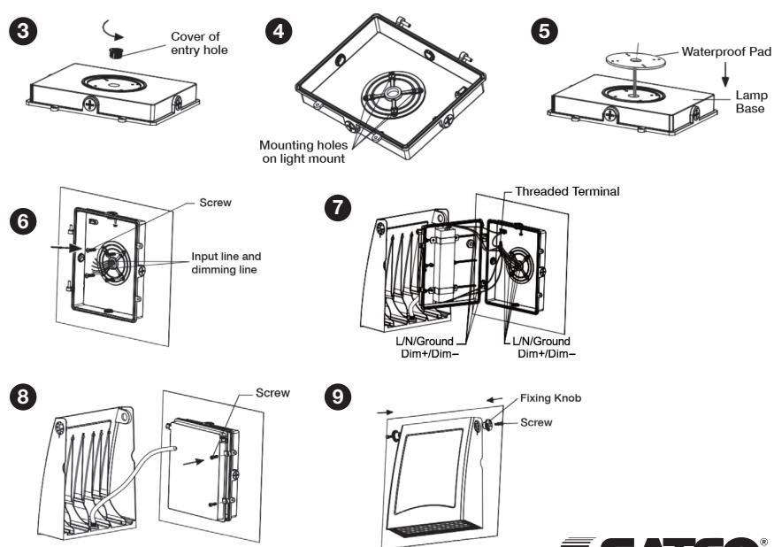
**STEP 4:** According to the embedded terminal box, punch the corresponding mounting hole on the light mount.
