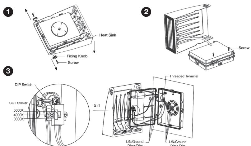
**STEP 2:** Remove screws with screwdriver, detach the cover from bottom box.
