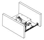
3 Suspended(T-bar) ceilings-extend bar hangers 1" past T-bars, then rest fixture on T-bars. Secure fixture to T-bars with wire.
