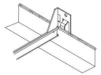
Junction box contains five (5) wires – 120-277V input & ground (white, black, & green) and 0-10V dimming (purple & grey). Make appropriate wiring connections per NEC and local code – 120-277V hot (black) to black, 120-277V neutral (white) to white, and ground (green) to green. If utilizing 0-10V dimming feature, wire dimmer + (purple) to purple and dimmer - (grey) to grey; otherwise, leave purple and grey wires capped. (See wiring diagram on page two.)
