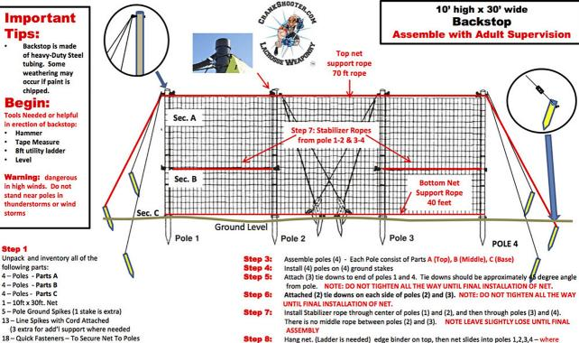
(3 extra for add'l support where needed 18 - Quick Fasteners - To Secure Net To Poles
