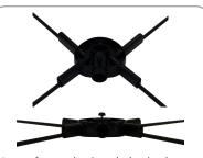
Insert four poles into holes in the hub. Make sure the poles are in all four arms of hub and through the holes opposite from the side with the thumb screw. 2
