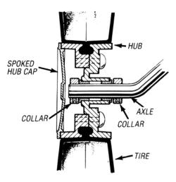
Hubcaps may also be fitted on the inboard face of the wheel, in particular the smooth hubcap, which nicely simulates the brake drum. To achieve this, the wheel should be off the axle and the hubcap snapped into the inboard face of the wheel. Use the axle hole as a drill guide to drill through the hubcap. Open out the hole to clear the inboard washer or collar.
