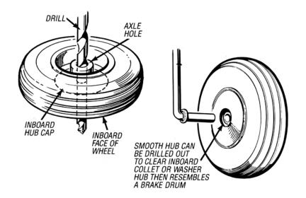
Hubcaps are a snap fit in place, but a hard landing has been known to displace them. To avoid loss apply a few spots of glue to the flange. Suitable glues are Pacer Plastic-Zap CA++, Testor's Plastic Cement, or RTV pipe cement as used by plumbers to join PVC pipes (available from the hardware store).
