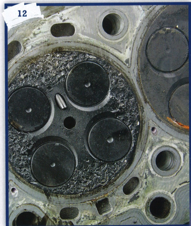
... and as you can see the damage to the cylinder head matches the piston quite well.
