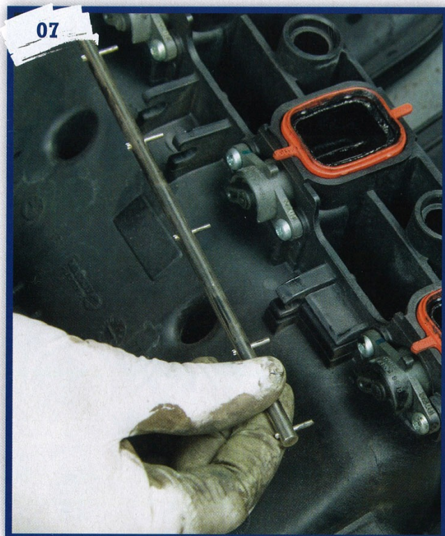
The swirl flaps are actuated by a rod that links them to a small servo. This can be removed and discarded.
