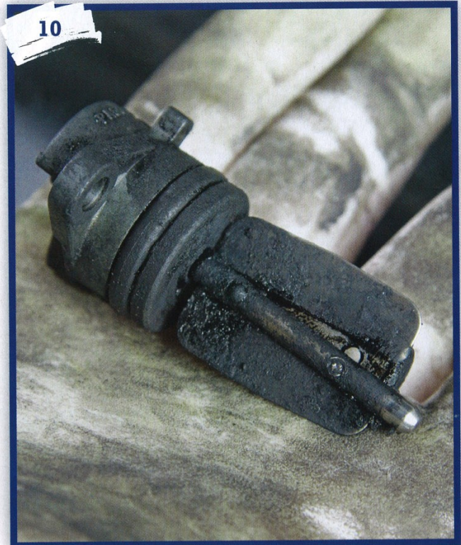
This is an example of a broken flap from a 320d engine. The consequences of this failure are shown in next two pictures.
