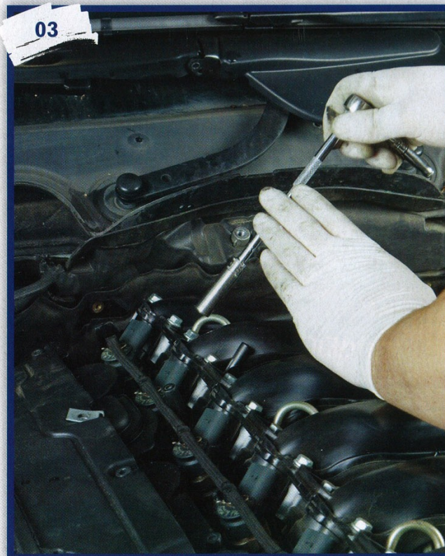
Remove the bolts which hold the manifold to the cylinder head.
