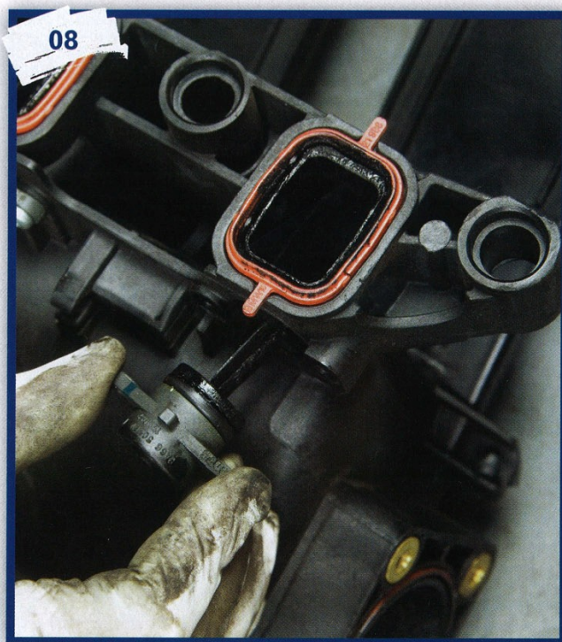
The swirl flaps are held into the manifold by two screws. After these are undone, the flaps can be withdrawn. Although they will be discarded, you might want to examine them to see if they were about to fail...
