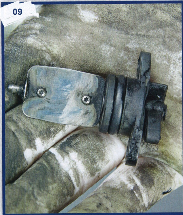
Note the two tiny screws which hold the flap to the spindle. They can work loose from vibration and just one of these sucked into the combustion chamber would write off the engine.
