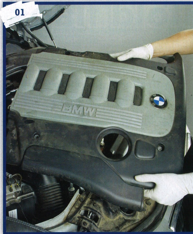
Remove the screws holding the elaborate plastic engine cover and lift it away to access the manifold.
