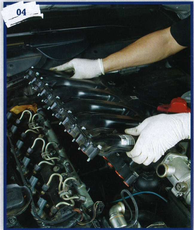
After loosening the EGR tube, the manifold can be removed. Don't let anything fall into the inlet ports!
