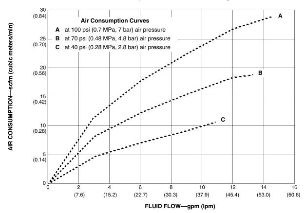
**To find Pump Air Consumption** (scfm or m³/min) at a specific fluid flow (gpm/lpm) and air pressure (psi/MPa/bar):
