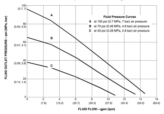
**To find Fluid Outlet Pressure** (psi/MPa/bar) at a specific fluid flow (gpm/lpm) and operating air pressure (psi/MPa/bar):
