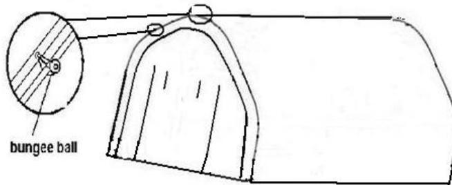
**5. Cover installation (inside of the cover with the pipe pockets facing down.)**
