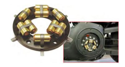
The base plate goes between a pressure plate and a diaphragm spring. You do not have to remove a spring. It can be slid through spring blades.
