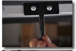
Screw mirror onto bracket. Tighten completely.
